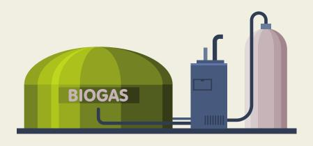
THE PURIFIED BIOGAS IS FED INTO A COGENERATION MODULE, WHERE IT IS COMBUSTED TO GENERATE ELECTRICITY AND HEAT.
